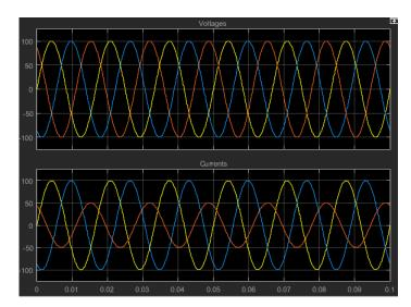
In this version of the model, one phase of the three-phase load has twice the resistance of the other two. Therefore, half as much current flows in that phase, as the second plot shows. However, because the load remains purely resistive, the voltage and current remain in phase with each other.
