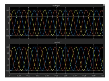
In this example, the **Component structure** parameter of the RLC block specifies that the electrical characteristics of the three-phase load are purely resistive. Therefore, for each phase of the three-phase system, the voltage and current remain in phase with each other. Because the resistance in each phase is  $1 \Omega$ , the magnitude of the phase voltage is equal to the magnitude of the phase current.
