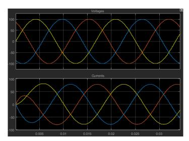
In "Build a Simple Three-Phase Model" on page 3-2, the electrical characteristics of three-phase load are purely resistive. In this model, the **Component structure** parameter of the RLC block is set to **Series RL**, meaning that the load has an inductive characteristic. The current flowing in each phase lags the voltage.
